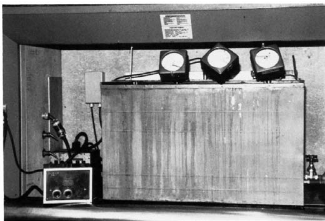
FIG. 1 Rotating Vessel Oxidation Test Apparatus
